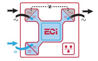
The ECI technology eliminates all single points of failure with full scalability; up to 32 modules in parallel and high efficiency of up to 96% in AC to AC conversion, and above 93.7% in DC/AC conversion, hence reducing operating costs. We can build the systems up to 1.35 MVA.
